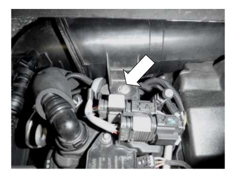
10. Using a flat-blade screwdriver carefully remove the sprung clip on the plastic coupler on intake pipe. Be very careful not to drop this sprung clip as it very difficult to retrieve it without taking the vehicle under trays off.
