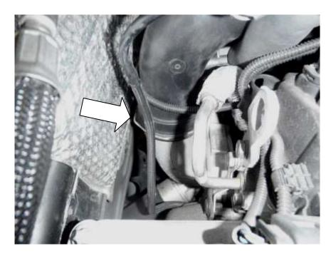
11. Using a flat-blade screwdriver unclip the wiring cable clip on the back of the plastic intake pipe (shown with the parts removed to illustrate).
