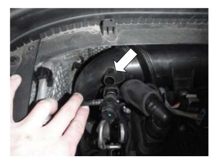
9. Using a T25 Torx driver undo 1x screw.
