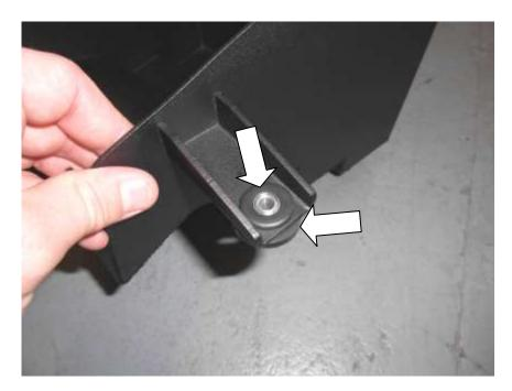
31. Carefully fit the airfilter tray in position and secure with the M6x20mm Allen bolt and 6mm penny washer.
