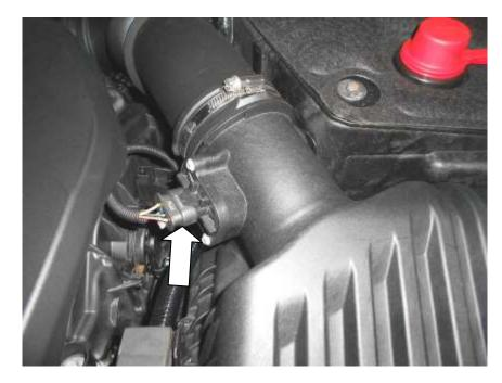
4. Using a 7mm Hose clamp driver or flat blade screwdriver undo the hose clamp.
