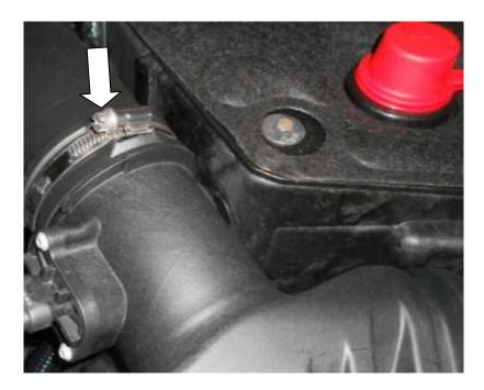
5. Using a 10mm socket, extension bar and suitable ratchet undo the bolt on the airbox bracket.
