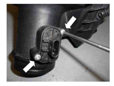
27. Using a T20 Torx driver undo the 2x screws and carefully remove the MAF sensor. Handle with care.
