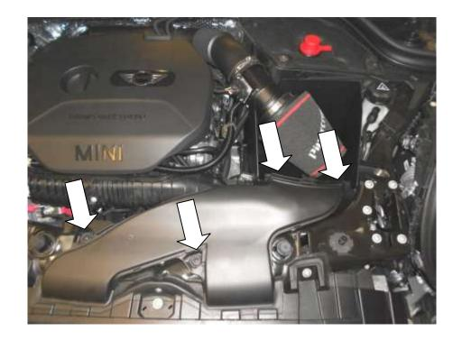
35. Refit the OEM ducting, using a 10mm socket secure with 2x nuts.
