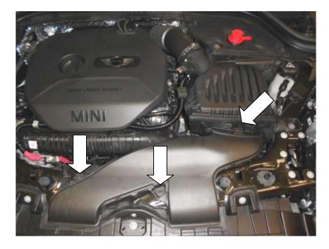
2. Using a 10mm socket, extension bar and suitable ratchet undo the 2x nuts. Unclip the intake duct where it meets the airbox and remove it from the vehicle.
