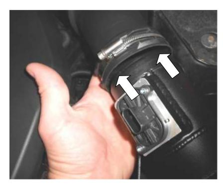
34. Reconnect the wiring to the MAF sensor.
