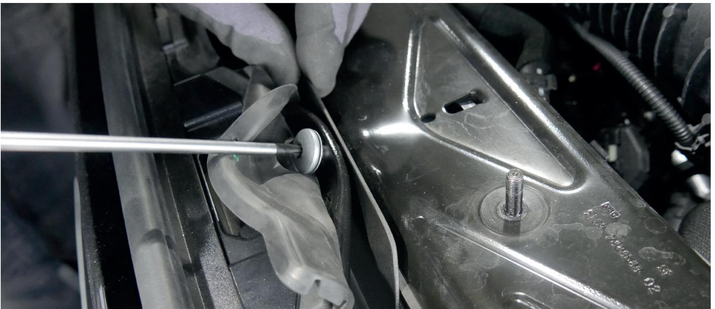
5. Mount the air collector and fasten it with the screws you removed earlier.
