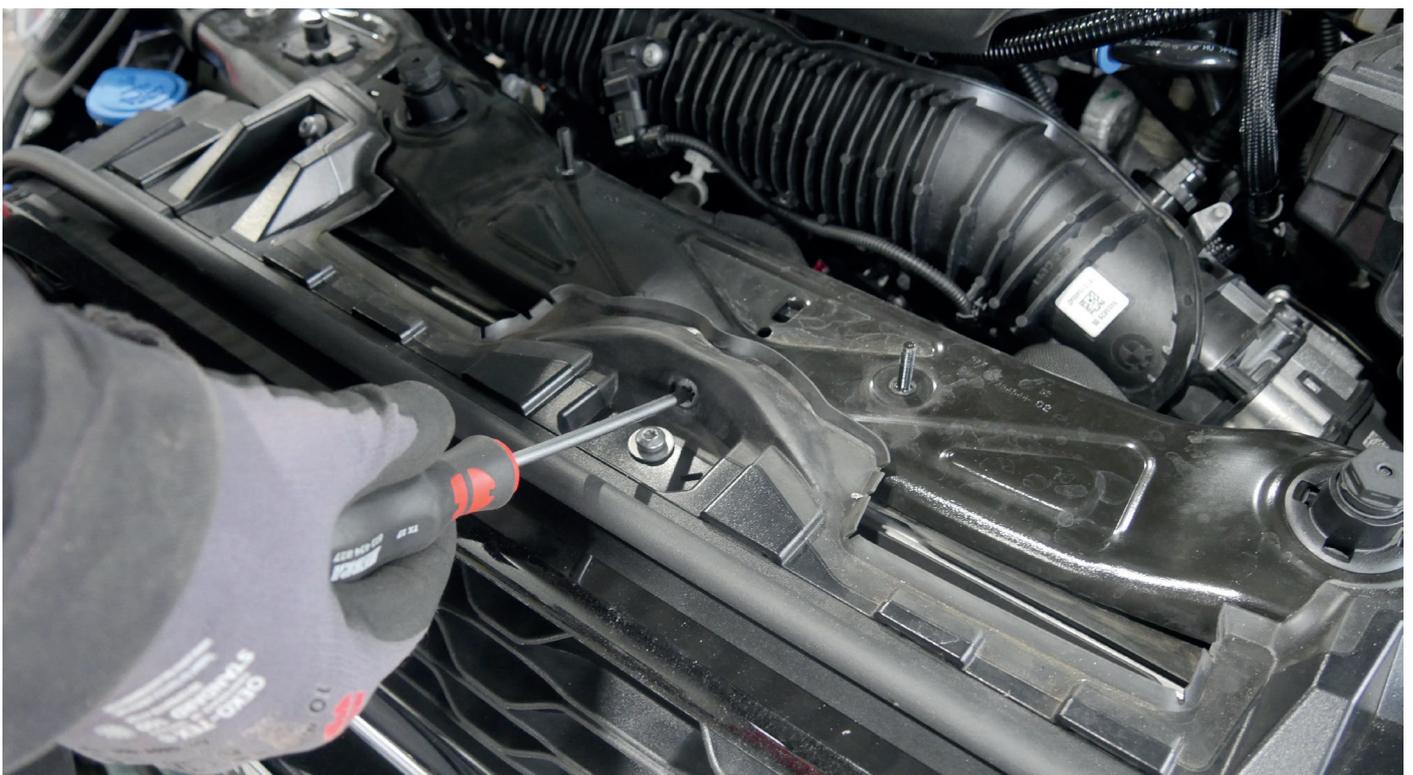
4. Now slide the air sheet between the front reinforcement and the lock bracket and fasten it with the screw you removed previously. Align the plate straight and tighten the screw firmly.
